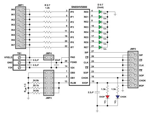
Figure 1. SN65HVS880 EVM Schematic
